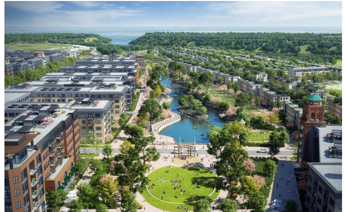
Figure 16. As part of the Ford Motor Assembly Plant redevelopment, the City of Saint Paul used Clean Water Funds to create a stormwater treatment system as part of a central water feature that filters stormwater runoff from more than 60 acres and removes 75% of phosphorus and 94% of total suspended solids (TSS) prior to discharging into the Mississippi River. This innovative biofiltration project, going above and beyond redevelopment standards, will clean 64 million gallons annually, preventing an estimated 145 pounds of phosphorus and over 55,000 pounds of total suspended solids from reaching the river while creating an amenity surrounded by green space that will provide multiple types of recreational opportunities for the community.
