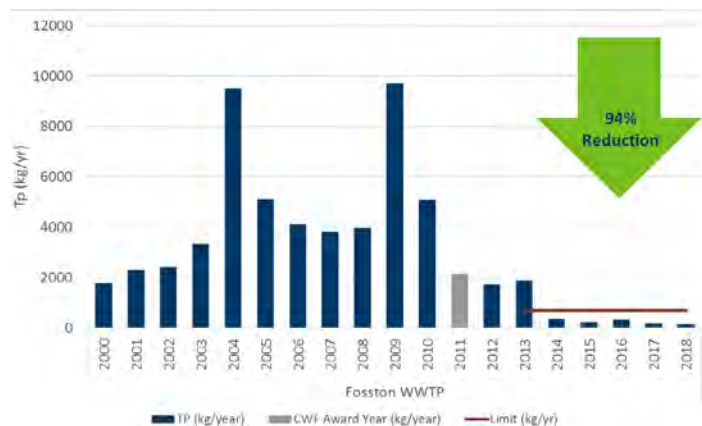
Figure 32. Total phosphorous reductions for Fosston Waste Water Treatment Plant
