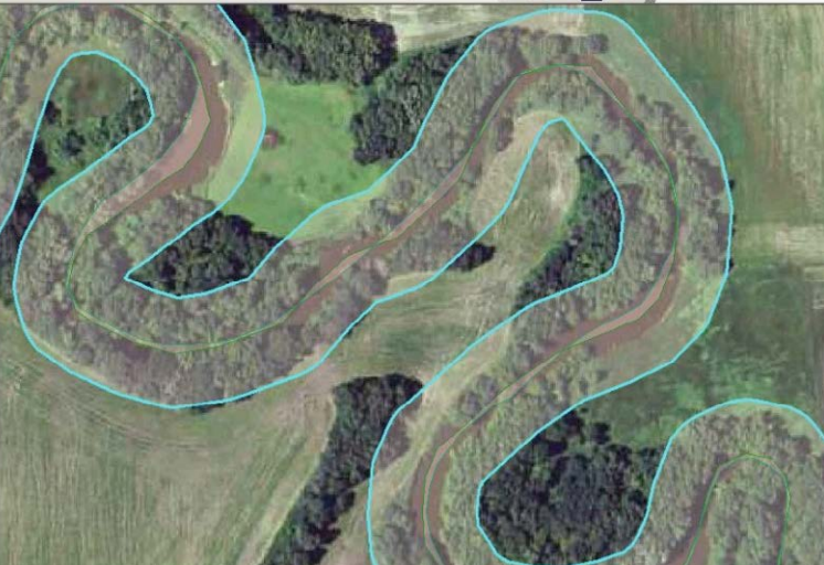
Lateral erosion calculation using aerial photography
