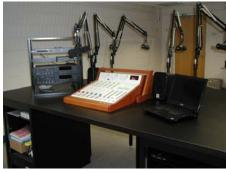
fashion, so as to make it possible to easily relocate it if necessary. The studio has a six-channel audio mixer, two CD players and an automation system. There are five microphones: the announcer mic and four guest mics. This studio can operate independently from KMSU, or can be the source for both KMSU and KMSK. This is the station's first step towards providing truly local arts and cultural programming for the Austin community rather than relying on having everything come out of Mankato.
