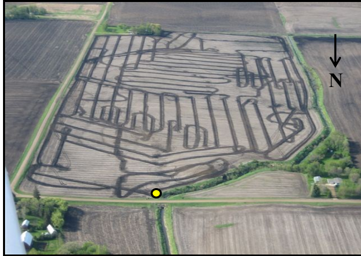
Figure 3.23: Modifications made to the BE2 watershed for monitoring the subsurface tile. Yellow dot indicates monitoring station location.
