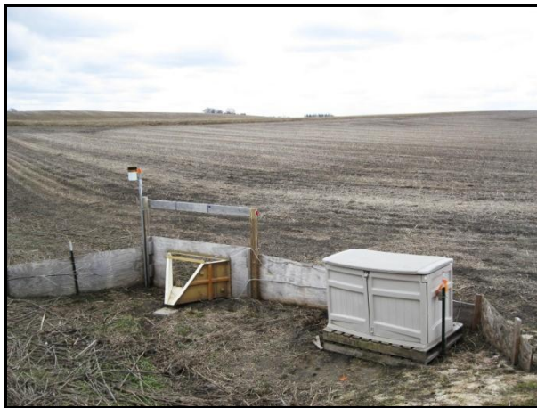
Figure 3.24: BE2 monitoring setup for overland surface runoff. Set up and equipment gifted from the Acetochlor Registration Partnership study.
