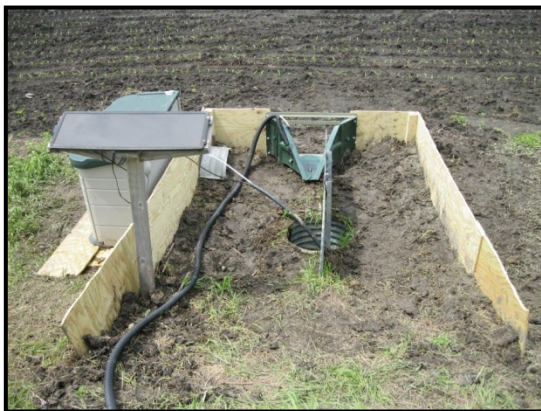
Figure 3.02: BE1 monitoring location showing 1.5 foot H flume, wingwall and open drop structure, May 2011.
